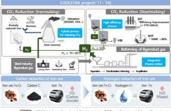
[Figure 4-13] Hydrogen reduction steelmaking
