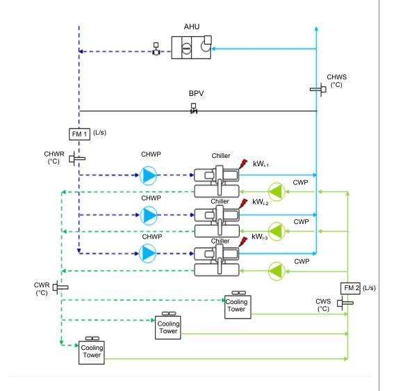
A:  $q_{evaporator}$  =  $m \times Cp \times \Delta T$  = FM1 x Cp x (CHWR - CHWS) B:  $q_{condenser}$  =  $m \times Cp \times \Delta T$  = FM2 x Cp x (CWR - CWS)
