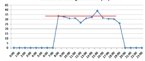
Based on the simulated building cooling load profile for the building operation hours from 8:00 to 19:00, the estimated most frequent occurring part-load condition of the installed capacity is 70%
