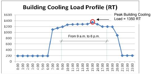
From the simulated building cooling load profile, the peak building cooling load is 1,350 RT (> 500 RT) and the minimum Design System Efficiency for water cooled chilled water plant is **0.70 kW/RT**.
