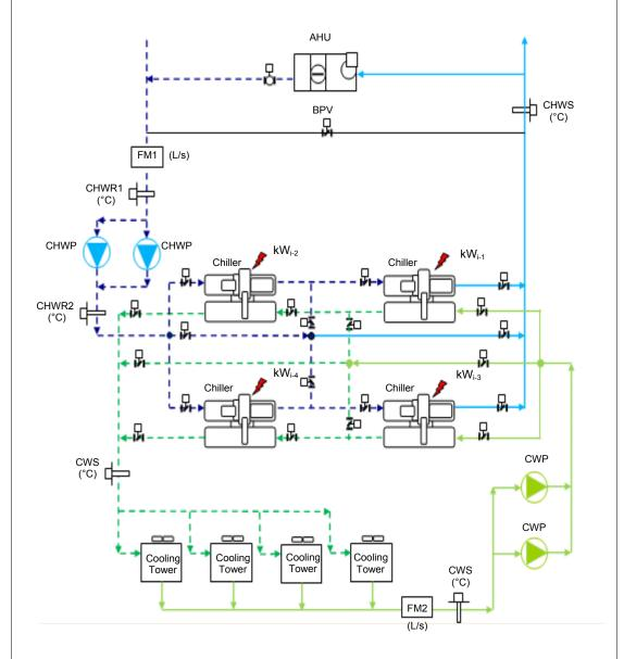
$\begin{array}{lll} \text{A:} & q_{\text{evaporator}} \\ \text{B:} & q_{\text{condenser}} \\ \text{C:} & W_{\text{input}} \end{array} \qquad \begin{array}{ll} = \text{FM1 x Cp x (CHWR2 - CHWS)} \\ = \text{FM2 x Cp x (CWR - CWS)} \\ = \text{kW}_{i\text{-}1} + \text{kW}i_{\text{-}2} + \text{kW}i_{\text{-}3} + \text{kW}i_{\text{-}4} \end{array}$
