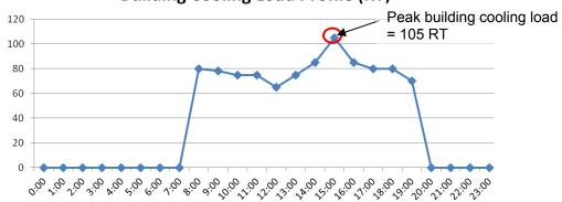
From the simulated building cooling load profile, the peak building cooling load is 105 RT (< 500 RT) and therefore the minimum Design System Efficiency for VRF system is **0.90 kW/RT**.
