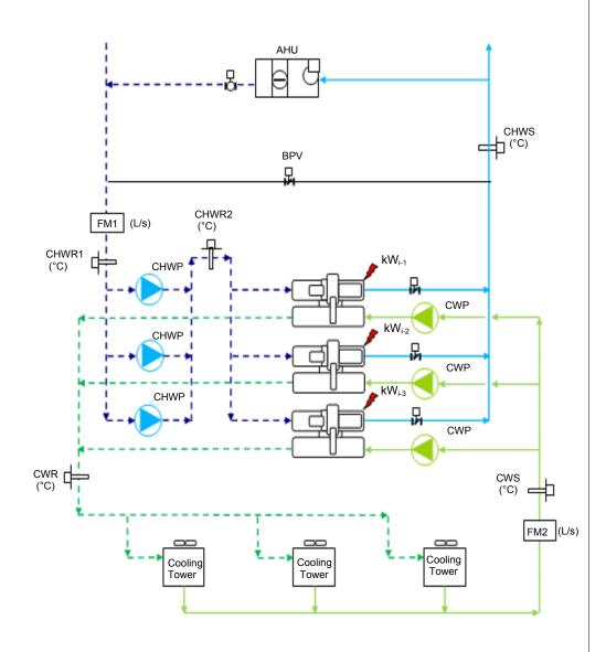
$\begin{array}{ll} \text{A:} & q_{\text{evaporator}} \\ \text{B:} & q_{\text{condenser}} \\ \text{C:} & W_{\text{input}} \end{array} \\ & = \text{FM1 x Cp x (CHWR2 - CHWS)} \\ & = \text{FM2 x Cp x (CWR - CWS)} \\ & = \text{kW}_{i-1} + \text{kWi}_{-2} + \text{kWi}_{-3} \\ \end{array}$
