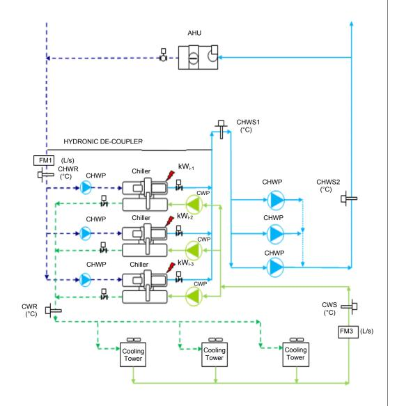
A:  $q_{evaporator}$  = FM1 x Cp x (CHWR – CHWS1) B:  $q_{condenser}$  = FM3 x Cp x (CWR - CWS)
