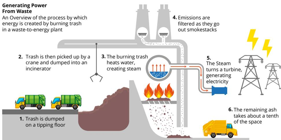
**Figure 6.4 Illustration of Waste to Energy process flow**
