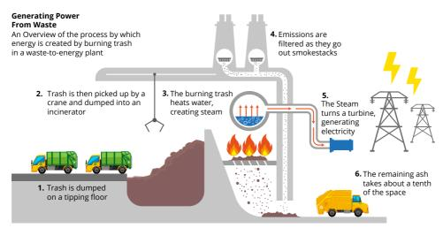
Figure 6.4 Illustration of Waste to Energy process flow
