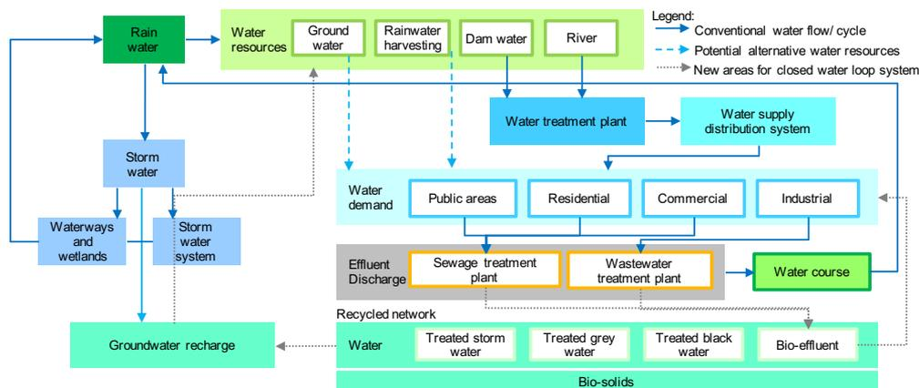
**Figure 7.3 IUWCM and closed water loop system<sup>6</sup>**
