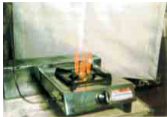
FIGURE 3 HYDROGEN COOK STOVE DEVELOPED BY BANARAS HINDU UNIVERSITY, VARANASI
