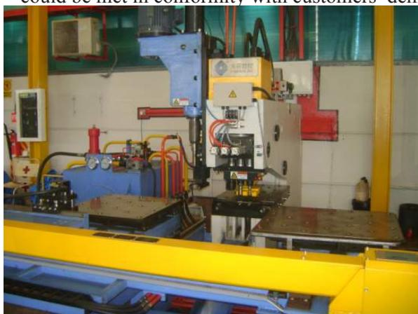
*Fully Automated CNC Angle punching Machine*
