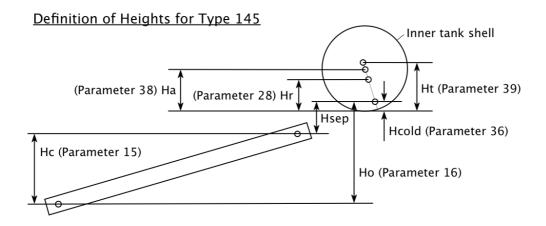
Note: If a dip tube is used on the cold inlet port then the measurements Hsep and Hcold are relative to the level of the outlet of the dip tube.
