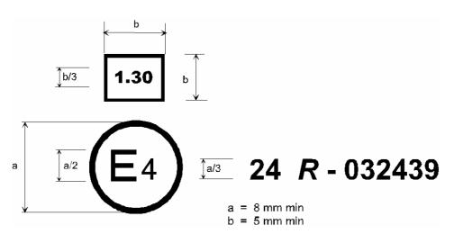
The above approval mark affixed to an engine/vehicle shows that, pursuant to Regulation No. 24, the engine/vehicle concerned has, with regard to the emission of visible pollutants by the engine, been approved in the Netherlands (E 4) under approval number 032439; the Regulation, at the time of approval, included already the 03 series of amendments. The corrected absorption coefficient is  $1.30 \text{ m}^{-1}$  (in the case of a vehicle approval).
