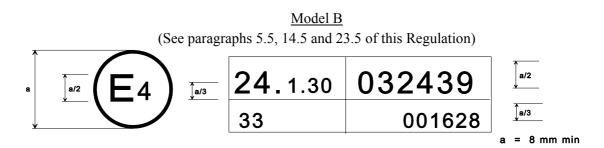
The above approval mark affixed to an engine/vehicle shows that the type concerned has been approved in the Netherlands (E 4), pursuant to Regulations Nos. 24 and 33.  $\frac{*}{}$  The approval numbers indicate that, at the dates when the respective approvals were given, Regulation No. 24 included already the 03 series of amendments, but Regulation No. 33 was in its original form.
