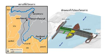
The Xayaburi hydro power project is a reinforce concrete dam with 810 meters long and 28.5 meters net water head. Ten floodgates were installed to produce electricity. Seven of 175 MW and one of 60 MW generators have been installed to generate electricity for sell to Thailand and Laos PDR., respectively. Total electric power generation is 1,285 MW and it can produce average 7,370 unit of electricity annually.
